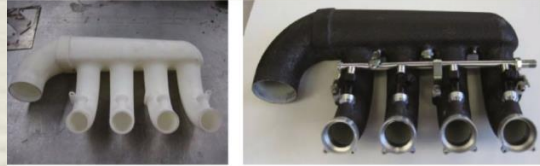
(a) Final assembly of an intake manifold fabricated by FDM; (b) completed intake system after a composite layup process and final assembly of sensors and mounts (Source: [166])
